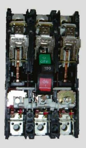
HPL Electric's Superior Series Current Limiting MCCB was developed with the latest technology for heavy duty usage: a magnetic trip unit for reliable quality tripping when short circuit occurs, repulse force for moving and fix contact construction, zero arc distance for the arc chute moulded in with thread nut for the case and cover and a long lasting BMC material for mounting, super mechanical and electrical strength.
